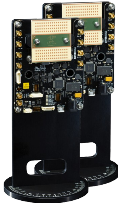
(b) The Siverts EVK06005 Phased Array, mounted with a Beamforming RF Module.
