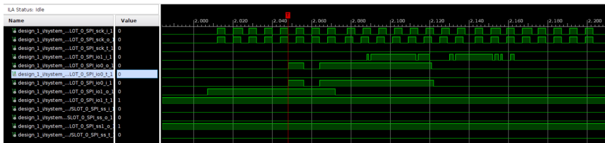
Figure 8: 1 Byte SPI read transaction on ZCU208, triggered by our driver going through the PL using EMIO. MOSI is referenced by io0_o and MISO by io1_i . We can count 24 SPI cycles, coherent with the EVK06005 specifications. The header access 0x00BF giving with read command 0b100 a command
