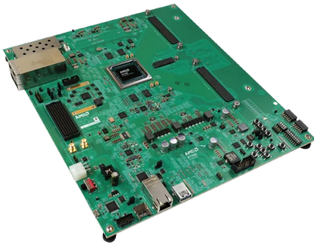
(a) The ZCU208 Evaluation Board without the XM655 Balun daughter card mounted for ADCs/DACs.
